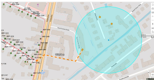
Figure 3 Distance measurement from mobile site candidate to the next junction in FNT GeoMaps
