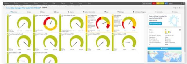
DCIM infrastructure health dashboard with temperature, humidity, and power consumption monitoring total and per individual power port.
