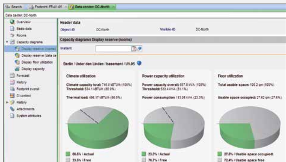
Capacity planning for power, floorspace, and cooling in FNT Command, including actual values and target values for specific days
