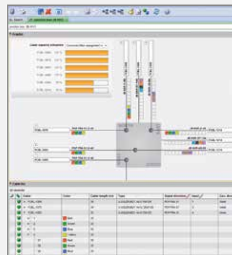
Junction box view and splice planning for precision capacity and allocation planning of services
